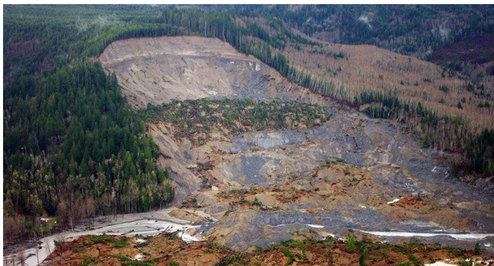
Fig. The cause of the destructive 2014 Oso, Washington landslide is believed to be a combination of excessive rainfall and logging which lead to liquefaction of the slope.
