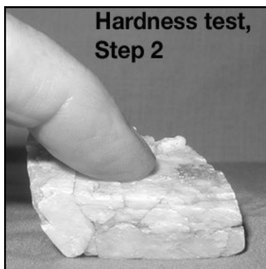
Rub the surface with your finger to remove the powder that has been formed.
