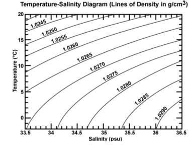
a) A sample of ocean water is taken and is determined to have a salinity of 34.5 psu and at the time of sampling had a temperature of 3°C. What density will the resulting sample have and how would this be determined using the graph above?
