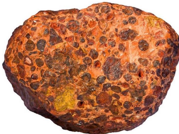
Natural scale (8 cm width) photo of a typical specimen of bauxite, comprising the reddish-brown iron oxides and the whitish clay kaolinite .
