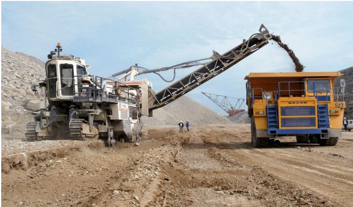
Open-pit mining: Selective mining of oil shale within limestone beds, Estonia ( http://mining-estonia.blogspot.com.au/ )
